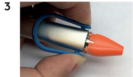
Squeeze the tool and pull off the tip cover.
