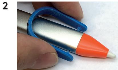
Align the tool with the two holes in the pencil tube.
