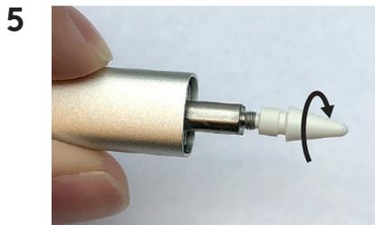
Insert new tip and twist clockwise to tighten securely.
