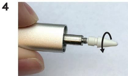
Twist the tip counter-clockwise to remove.
