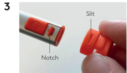
Align new cap to the top of the pencil tube.
